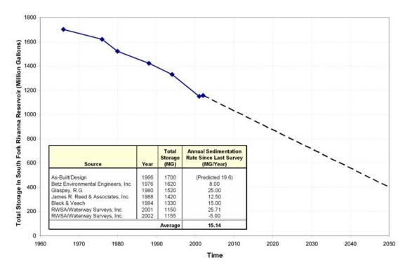
Figure 1: Plot Showing Change in Total Storage Over Time Due to Sedimentation at SFRR
